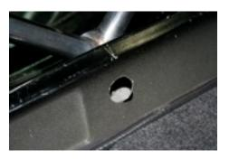
Switch back to the 3/8 and drill completely through both layers of the body.
