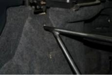
2. The hardest step is laying out and making the side holes in the carpet at just the right place. They are about 4" directly below the seat latch. And 30-1/2" forward from the welded stud that sticks out next to the taillight. Might be best to start by poking a screwdriver just to verify position. You will also need to cut through or remove the insulation pad behind the carpet so that it is out of the way. There is a little tolerance there, it is carpet and mostly hidden in
